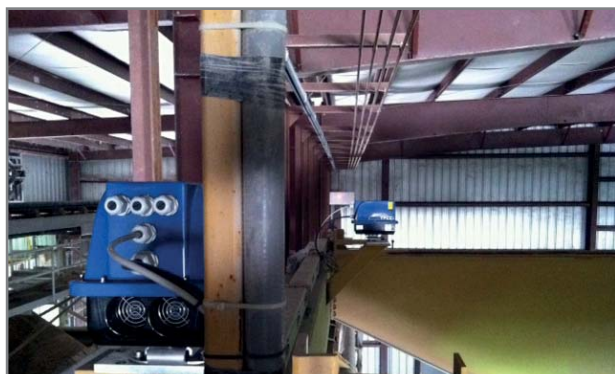
On left: TPCC® used on the bridge crane after modernization
