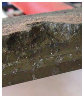
*Broken-out parts of a wearing strip section*
